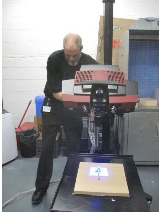
Figure 8 - Engineer using the GOM Atmos Triplescan Unit
